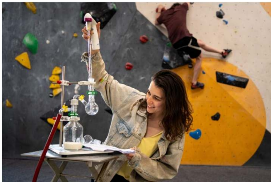
Anya Sherman uses an impinger (particle measuring device) to collect particulate matter from the air in bouldering gyms in Vienna. (Photo: Aaron Kintzi/CeMESS)
